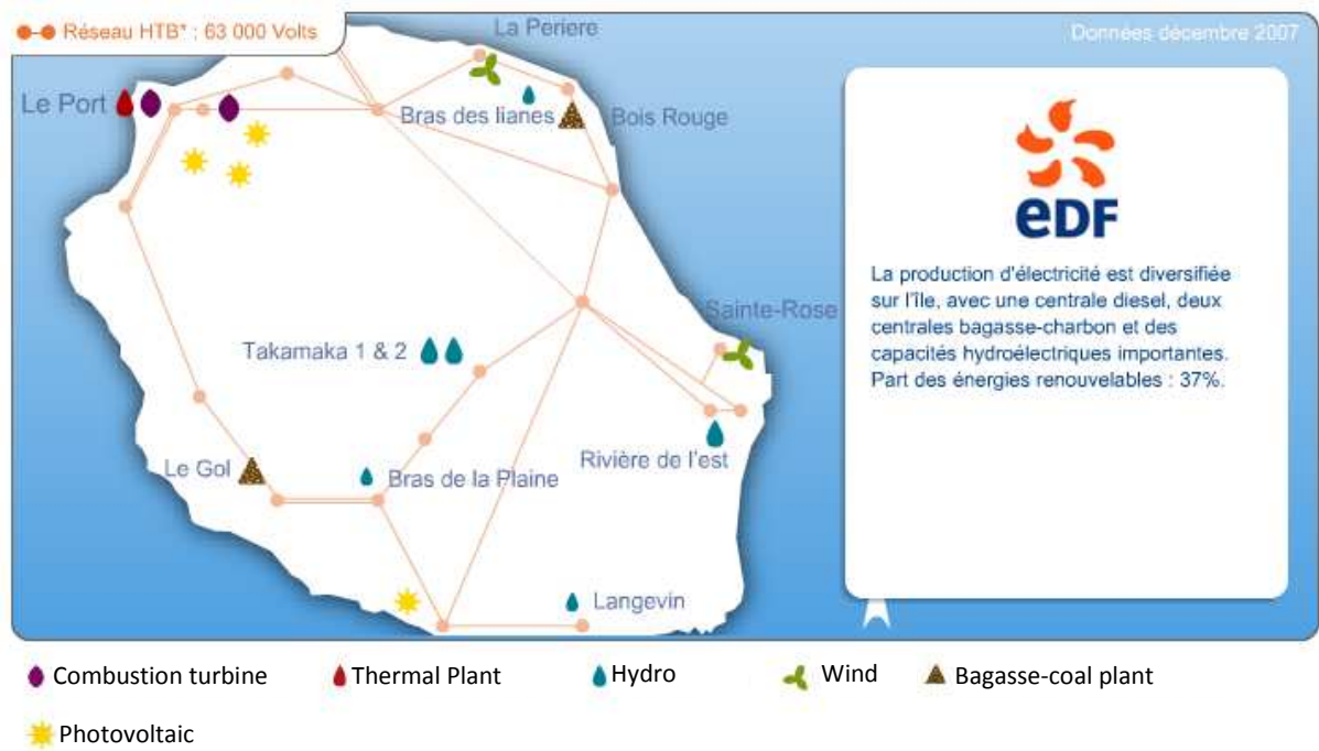
Figure 3 Power network of Reunion Island. The installed photovoltaic capacity was 1.3 MW in the South and 1.75 MW in the North in 2007. Source : sei.edf.fr
